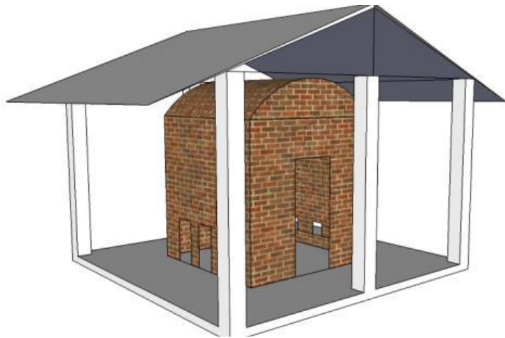
Figure 6: Kiln for the production of fired bricks
